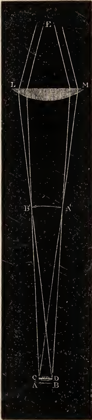
Diagram of simplest form of Compound Microscope.
